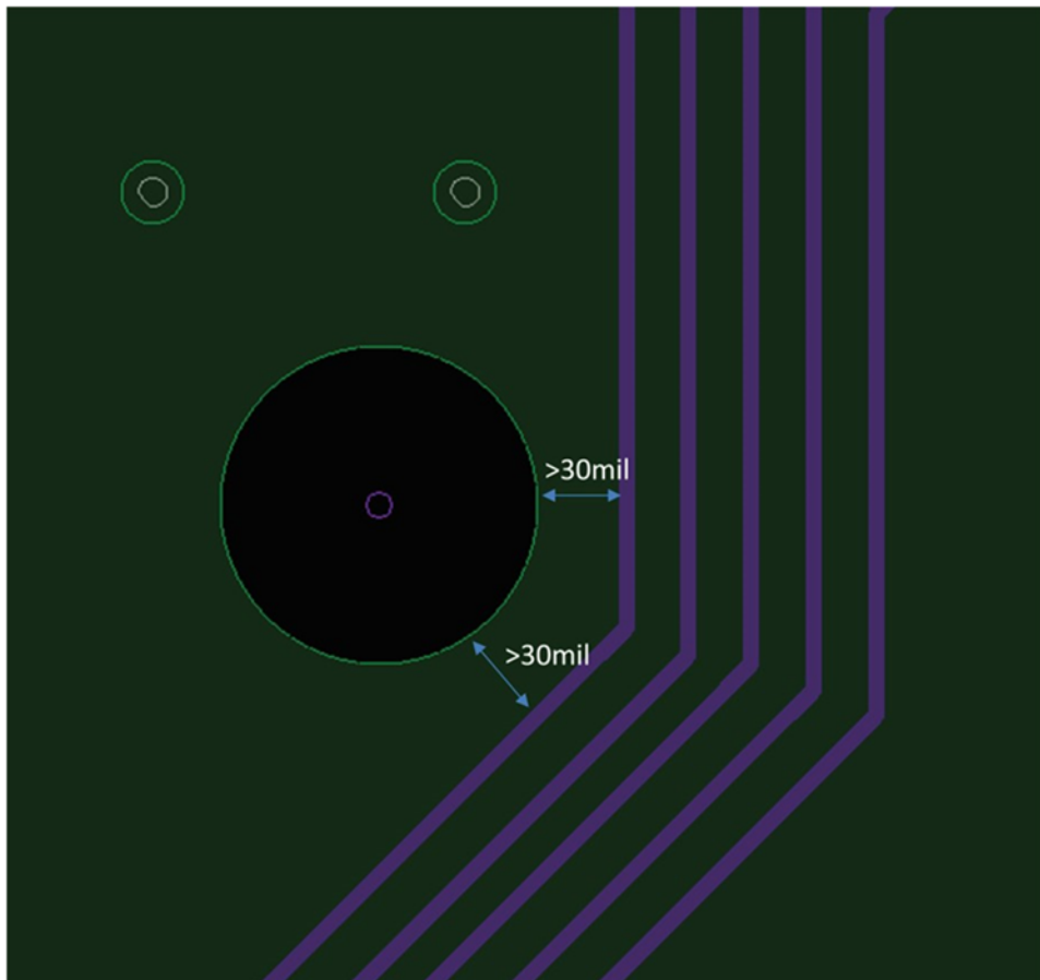
Figure 16: Signal Routing Over Solid Reference Plane
