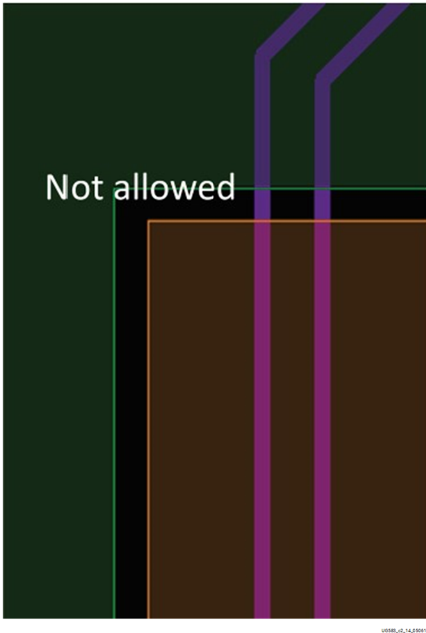
Figure 17: Signal Routing Over Reference Plane Split
