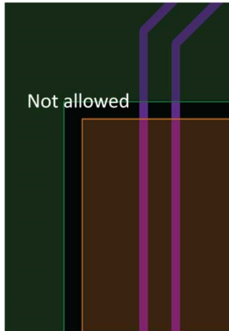
Figure 91: Signal Routing Over Reference Plane Split
