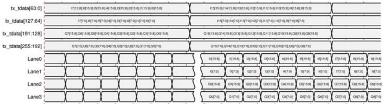
Figure 12: 64B66B Encoding - 4 Lane DAC, Frame size (F) = 1, 16 Bit I and Q with I Sample in Lanes 0 & 1 and Q Sample in Lanes 3 & 4
