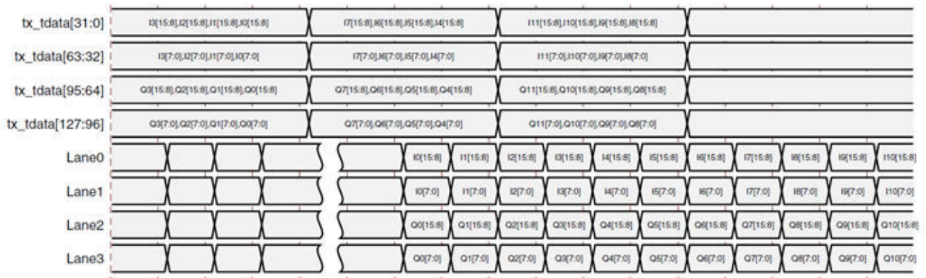
Figure 11: 8B10B Encoding - 4 Lane DAC, Frame size (F) = 1, 16 Bit I and Q with I Sample in Lanes 0 & 1 and Q Sample in Lanes 3 & 4
